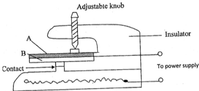
**Two metal plates A and B are riveted to form a bimetal strip as used above.**
