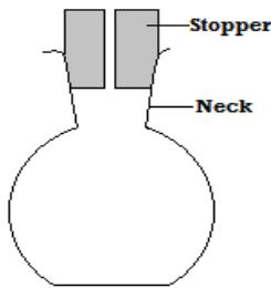
**N/B** Density bottle is used measure the density of either liquid or solid.
