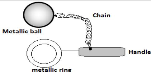
Observation: When the ball is heated, it does not pass through the ring but when it is left on the ring for sometimes it passes through. Explanation: When heated, the ball expands and so cannot go through the ring. When it is left on the ring for some time the temperature of the ball decreases and the ball contracts. At the same time the ring absorbs some heat from the ball its temperature increases and so it expands allowing the ball to pass through.
