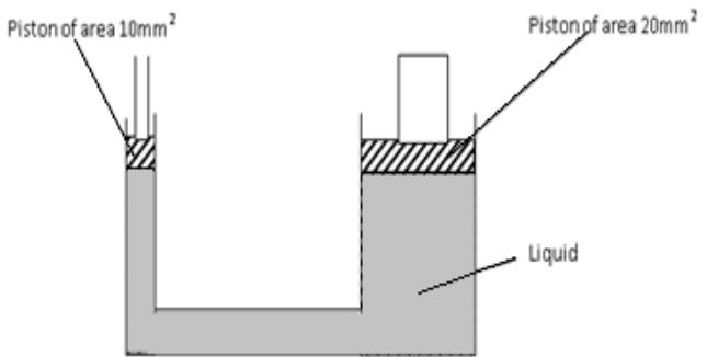
The two pistons are of areas  $10 \text{ mm}^2$  and  $20 \text{ mm}^2$  respectively. A force of 100N is applied on the smaller piston, find the load that can be lifted on the larger piston if:
