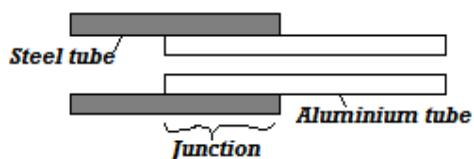
Explain how the two tubes can be separated by applying a temperature change at the same junction given that aluminum expands more than steel for the
