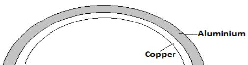
When temperature increases above room temperature aluminum expands at a faster rate than copper.
