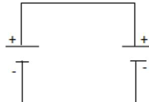
**Note:** Cells should be arranged in parallel only when they have the same e.m.f otherwise one will drain the other.
