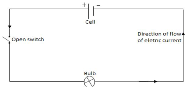
**Direction of the Flow of Electric Current**
