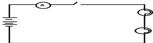
**Note:** Bulbs in parallel arrangement light brighter than those in series arrangement.
