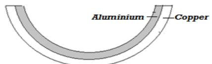
When temperature decreases below room temperature aluminum contracts at a faster rate than copper.
