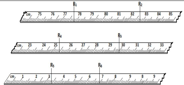
$$R_1 = 77.9 \text{ cm}, R_2 = 82.8 \text{ cm}, R_3 = 25.5 \text{ cm}, R_4 = 30.0 \text{ cm}, R_5 = 3.4 \text{ cm}, R_6 = 7.0 \text{ cm}$$
