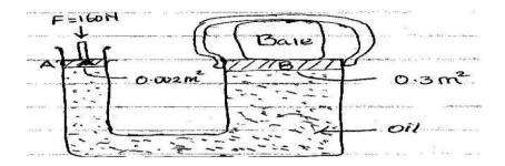
If aforce of 160N is applied on the small piston. Determine:
